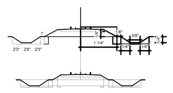
This is an illustration of the ballast and drainage as set by the SOO Line Standards Vol.1
